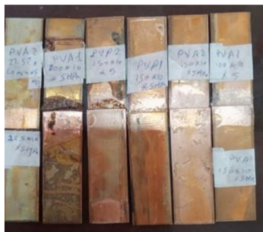
Figure 3: Manufactured copper samples to place the adhesive between them.
