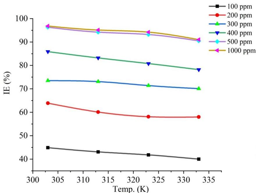
**Figure 3.** Inhibition efficiency plotted against temperature.
