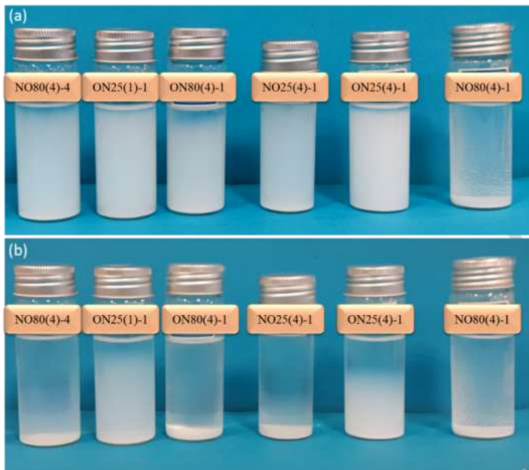
Figure 3. Nanostructure stability in water after (a) 1 st day, and (b) 10 th day.
