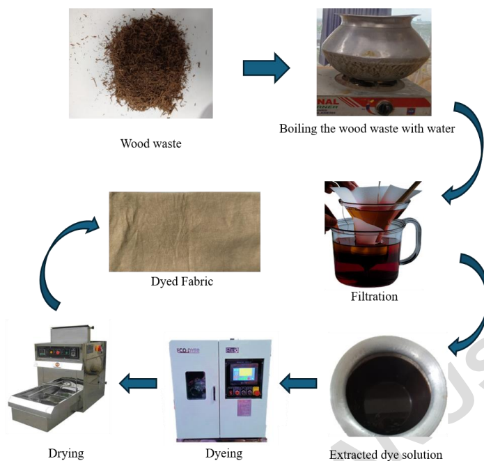
Figure 1. Process sequence for dyeing cotton fabrics using Dalbergia sissoo wood waste.
