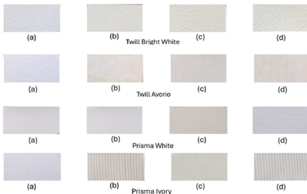
Figure 1: Image of uncoated (a) and coated recycled paper boards with RSF (b), WSF (c) and CSF (d) formulations.
