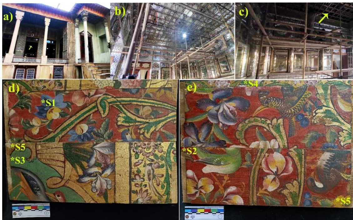
Figure 1: a) Sadr Jahromi's house in Shiraz, b and c) wooden panel painting discovered under mirrorwork during ceiling restoration, d and e) wooden panel painting of Sadr Jahromi's house and sampling locations, S1: Blue, S2: Red, S3: Green, S4: Yellow, S5: Metal leaf and substrate, S6: varnish.
