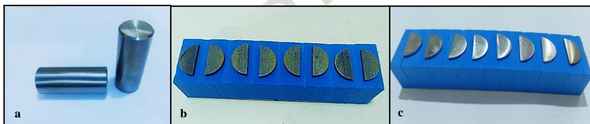
Figure 2: a) \text{Ti}_6\text{Al}_7\text{Nb} alloy rod as received, b&c) samples before and after grinding.
