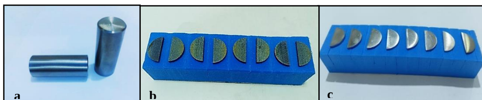
Figure 2: a) Ti6Al7Nb alloy rod as received, b and c) samples before and after grinding.
