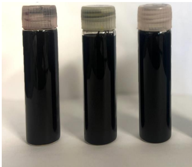
Figure 5: Photographic images of the graphene dispersions: (left) SDBS-0.75-MS, (middle) SDBS-0.25-MS, and (right) SDBS-0.10-MS.
