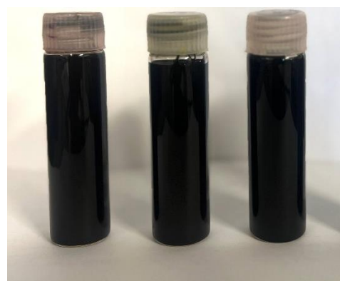
Figure 5: Photographic images of the graphene dispersions: (left) SDBS-0.75-MS, (middle) SDBS-0.25-MS, and (right) SDBS-0.10-MS.
