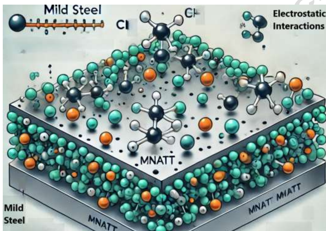
Figure 10. Schematic Representation of the Physisorption-Based Corrosion Inhibition Mechanism of MNATT on Mild Steel in 1 M HCl.
