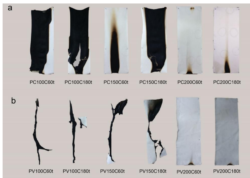
Figure 1: Polyester/cotton (a) and polyester/viscose samples (b) after direct flame test.
