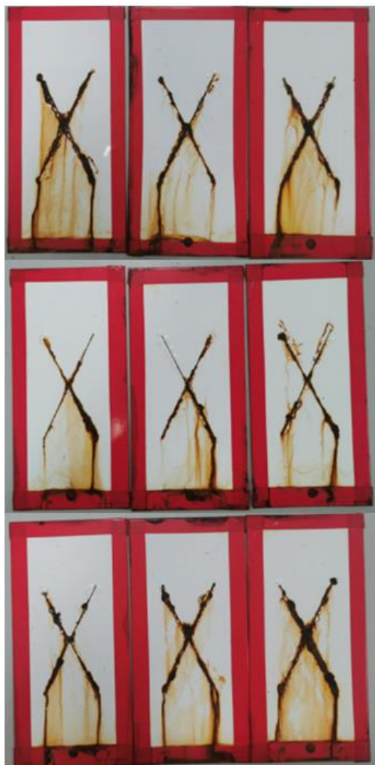
Figure 8: Corrosion progression after salt spray test for the coated plates. Top: UT (PVC: 13%), Middle: TT3 (PVC: 13%), and Bottom: TT3* (PVC: 11%).
