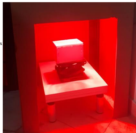
Figure 3: Schematic of the apparatus developed for exposure to NIR radiation and a sample thermogram [This figure was prepared by the authors].
