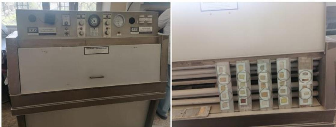
Figure 2: QUV tester and the samples inside it.
