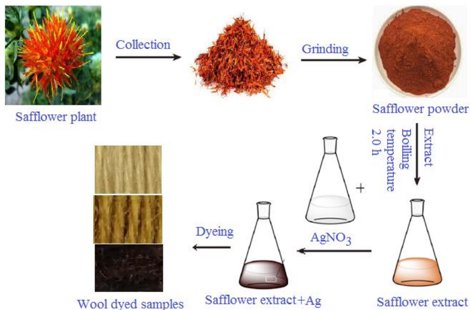
Figure 1: Scheme of Ag NPs synthesized on the wool by safflower extract.
