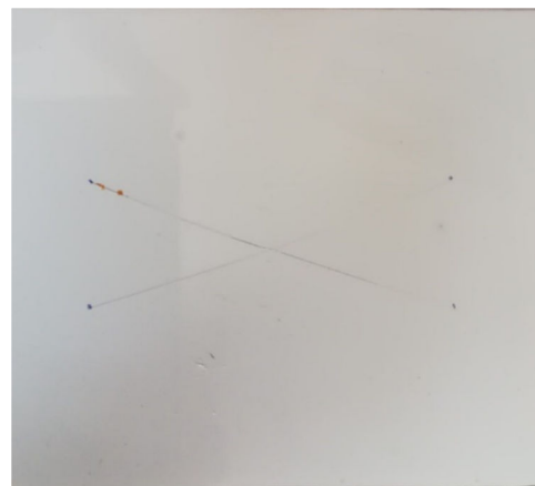
Figure 6: Salt Spray test for steel substrate coated with PU-E within 120 days.
