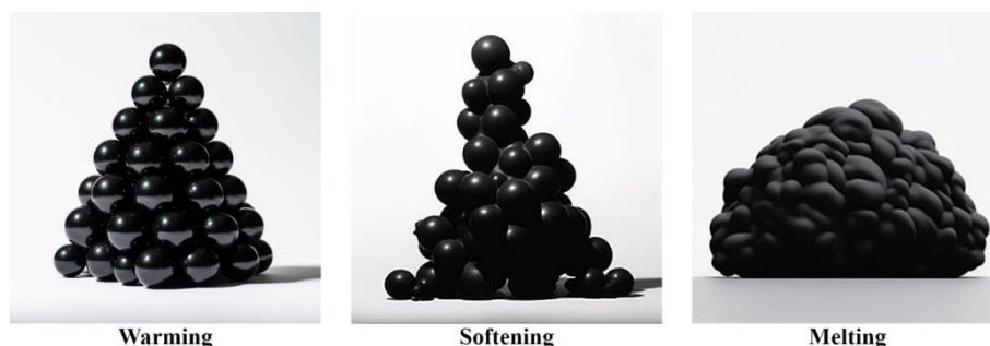
Figure 4: Schematic illustration of the fusing stages of toner in electrophotographic printing.
