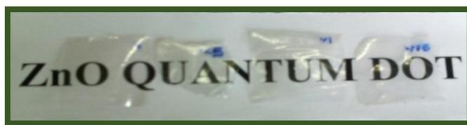
**Figure 12:** The image of transparency of the epoxy/ZnO QD nanocomposite films.
