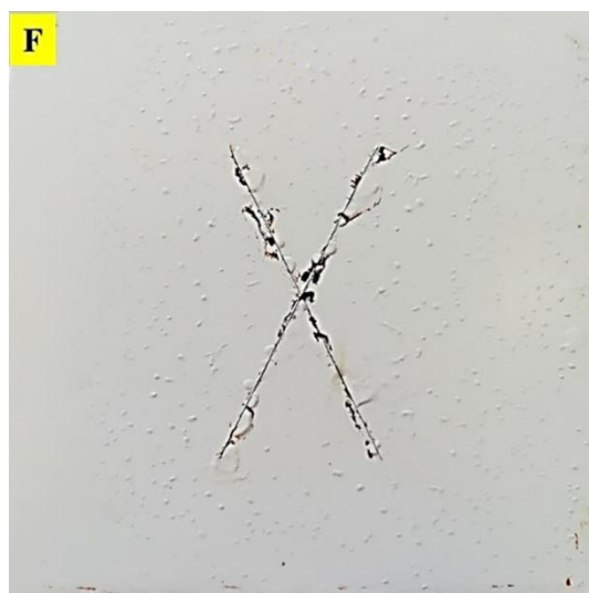
Figure 9: Salt spray test for FEVE coated steel for 360 hours.
