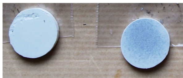
Figure 4: Left: Annealed sample “950”, right: as-sintered sample “950”.
