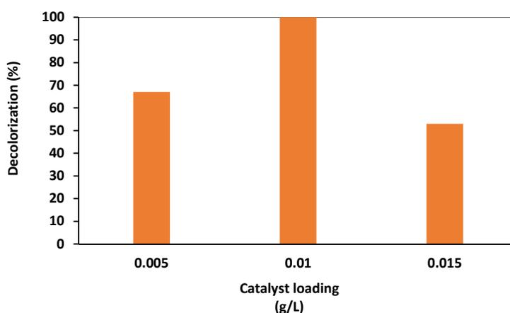
**Figure 5:** Effect of ZnO/W photocatalyst loading on decolorization efficiency, Reaction conditions: dye concentration 20 mg/L and pH=5.
