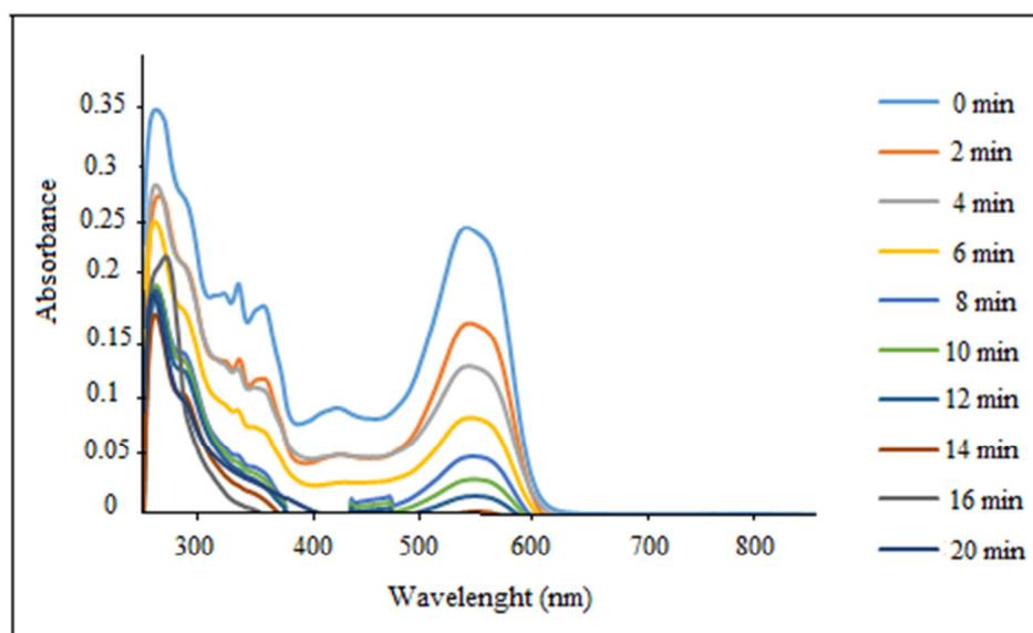
Figure 2: UV-Vis Spectral change for the degradation of 20 mg/L RR31 by ultraviolet light at different time.
