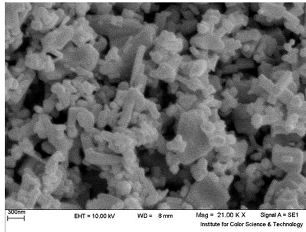
**Figure 3:** Scanning Electron Microscopy (SEM) of ZnO/W.
