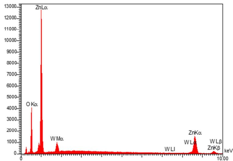
**Figure 4:** Energy Dispersive X-ray (EDX) spectra of ZnO/W.
