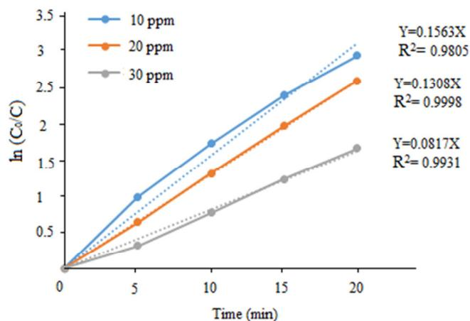
**Figure 8:** Kinetic study of RR 31 decolorization with different dye concentrations. Reaction conditions: catalyst loading 0.01 g/L, and pH=5
