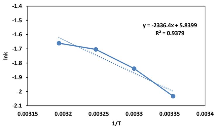
**Figure 9:** Arrhenius activation energy plot for kinetic study.
