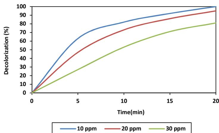
**Figure 7:** Effect of initial dye concentration on decolorization of RR 31 by ZnO-W photocatalyst reaction conditions: catalyst loading 0.01g/L and pH=5.
