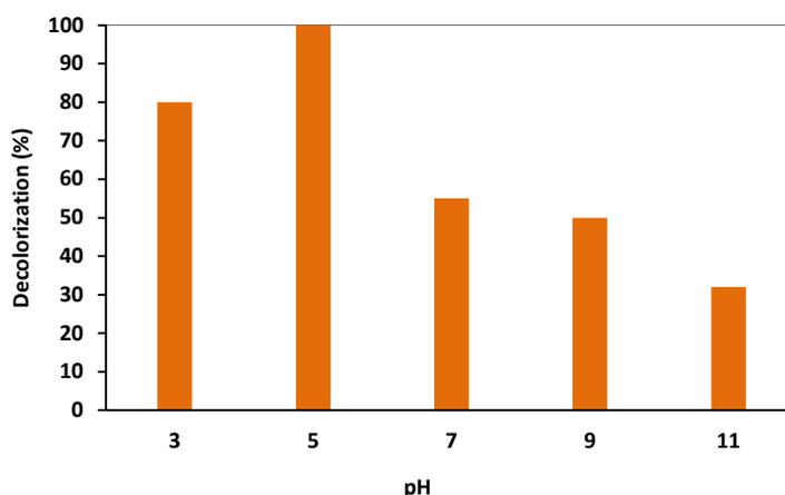
**Figure 6:** Effect of pH on decolorization of RR 31 by ZnO-W photocatalyst reaction conditions: catalyst loading 0.01 g/L, dye concentration 20 mg/L.
