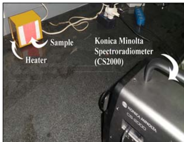
Figure 3: Arrangement of sample, heater and spectroradiometer.
