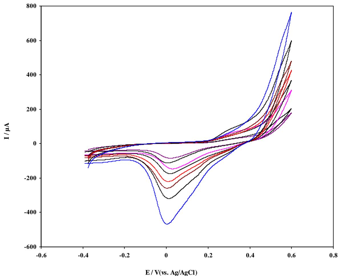
**Figure 5:** CVs of the biosensor in PBS ( $0.1\text{M}$ ,  $\text{pH}= 7.0$ ) at various scan rates. The scan rate (from inner to outer) is 10, 20, 40, 60, 80, 100, 150 and  $200\text{ mVs}^{-1}$ , respectively. Inset: plot of currents versus scan rate.
