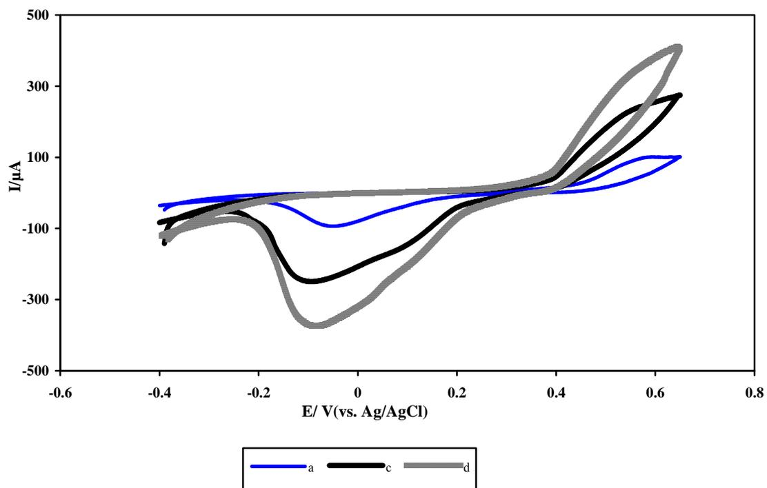
**Figure 4:** (a) Cyclic voltammograms of the biosensor without, with glucose (40mM), (b) glucose (80mM) and (c) in PB solution (0.1M, pH= 7.0) at scan rate of  $20\text{mV/s}$ .
