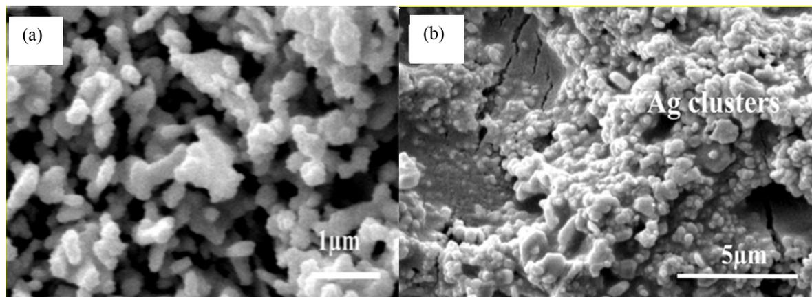
**Figure 2.** The SEM image of inkjet deposited silver pattern on paper substrate with AAAG protocol (X5000). The SEM image of same sample after hot press at 150 °C for 20 second and cleaning with double distilled water(X15000).
