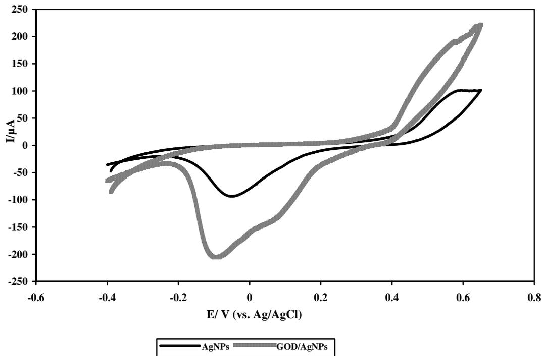
**Figure 3:** Cyclic Voltammograms of AgNPs/paper (a), and GOX/AgNPs/paper (b) electrodes in 0.1M PBS solution (pH=7.0) at  $20\text{mVs}^{-1}$ .
