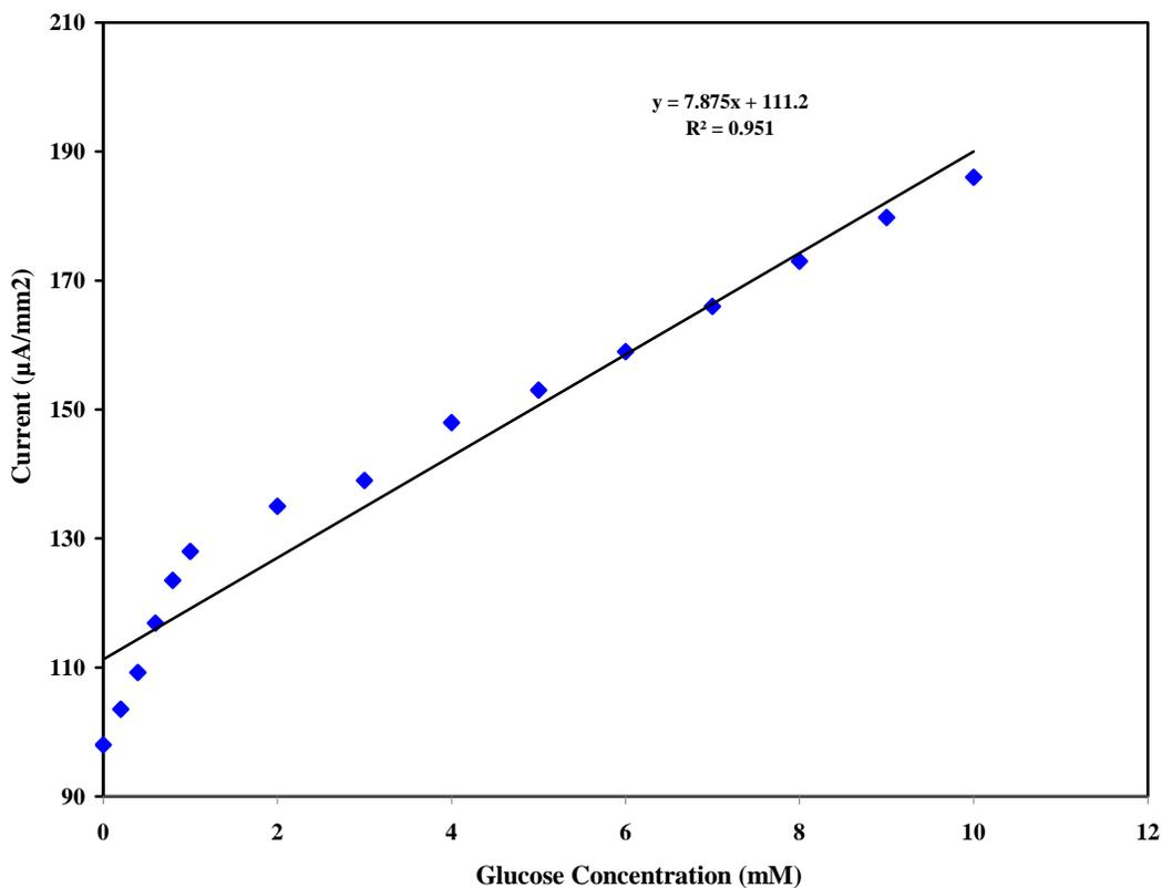
**Figure. 6:** The calibration curve ( $R^2= 0.951$ ) corresponding to amperometric responses at -0.4 V to 0.65V. Scan rate:  $20\text{mVs}^{-1}$ .
