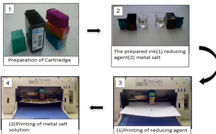
Figure 1. The steps of inkjet printing by reducing of silver nanoparticle on paper substrate.
