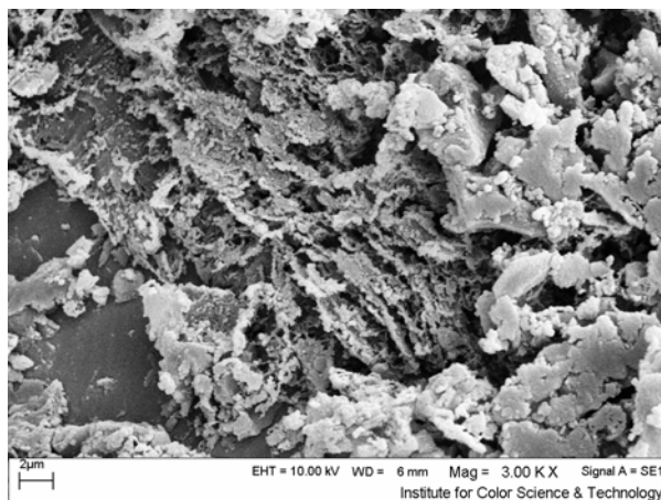
Figure 1: SEM images of the synthesized Cl-DPP at equal ratio of [BMIM][OH] and [BMIM][BF 4 ] in the absence of sodium t -amyl oxide.
