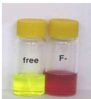
Figure 4: The yellow to deep purple color of AFTN change upon titration with F^- .
