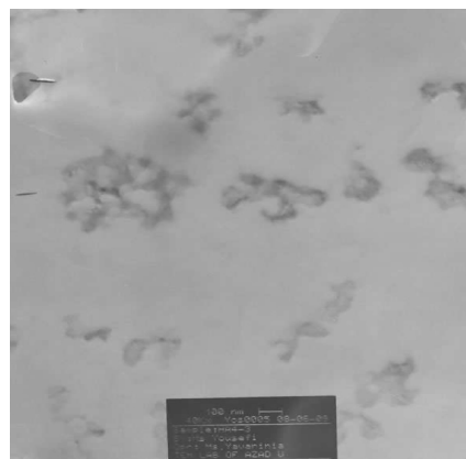
Figure 10: Morphology of HA4 hybrid resin.
