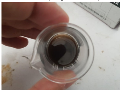
GO + STARCH after sonication in THF for 5 minutes (Amplitude 20%)
